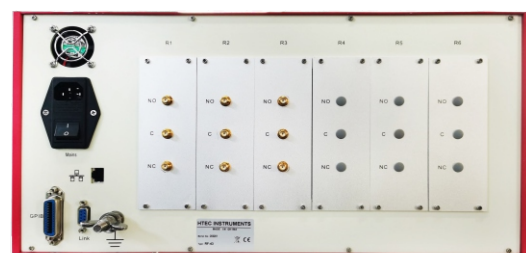
Rear view of Relay Switching Unit
